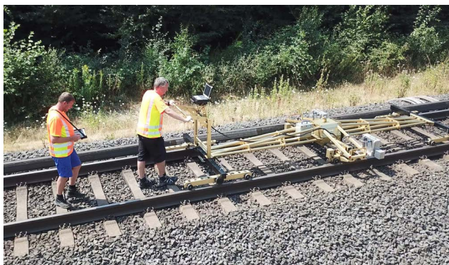
Measuring the track geometry using the EMA uni
