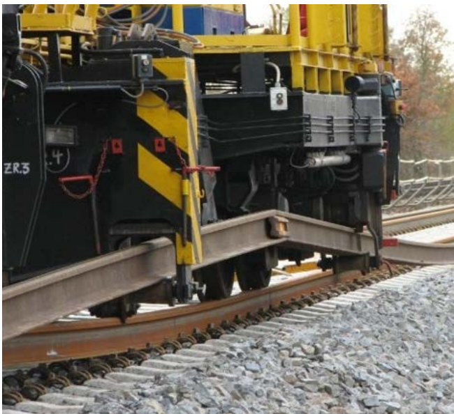
SWW 1 and SWW 2 Rail Replacement Wagons: designed for assembly-line rail replacement
