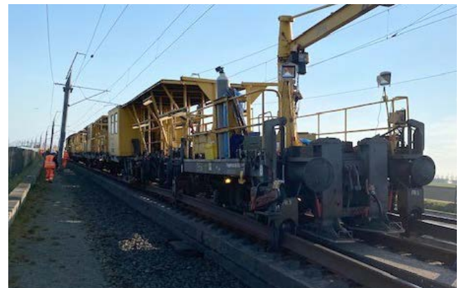
SWW 1 and SWW 2 Rail Replacement Wagons: designed for assembly-line rail replacement
